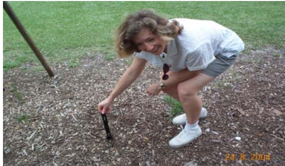
Figure 90. Checking the depth of loose material.
